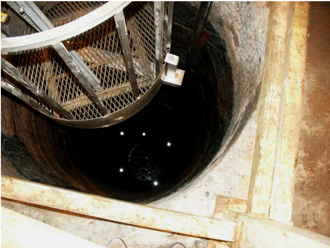
Figure 2-2. Laser scanning of a vertical deposition hole performed by Berg Bygg Konsult AB. The laser scanner (not shown in the picture) had to be mounted up side down under the lift cage.
