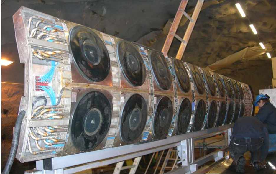
Figure 4-2. New water cushions being installed under the water cushion palette.
