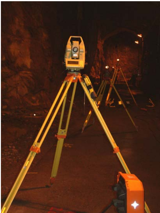
Geoiden AB surveying reference points to be used later when laser scanning takes place.
